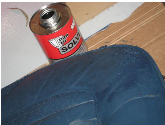
TOP AND BOTTOM - THE OLD DYE LOOSENS WITH THE AID OF THE SOLVENT WHICH MAKES IT EASY TO SCRAPE OFF
