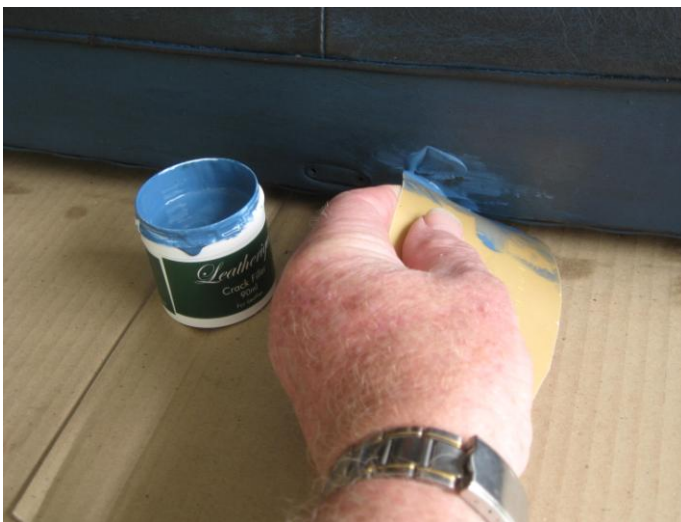
CRACK FILLER BEING USED TO FILL AN UNWANTED HOLE
