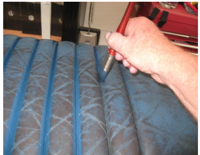
USING A FINE BRUSH TO MAKE CERTAIN THE DYE PENETRATES THE STICHING IN THE PLEATS AND PIPING
